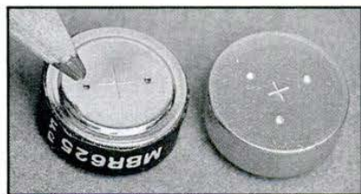
Holey Moley! Prototype Wein cell (left) has only two air holes; zinc-air hearing aid batteries have three or four. Why? Fewer holes mean less evaporation of moisture, so cells can last longer (see text).
