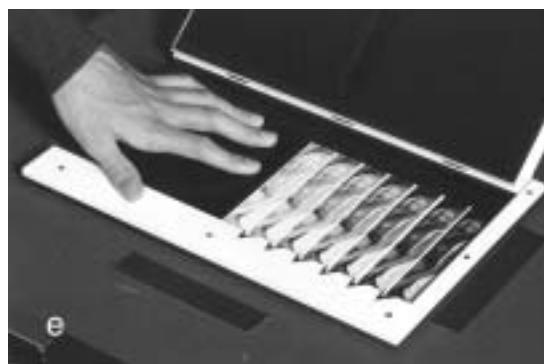
fig.2a-e An localized test strip is the best choice, if the governing highlights are concentrated in a relatively small area of the image.
