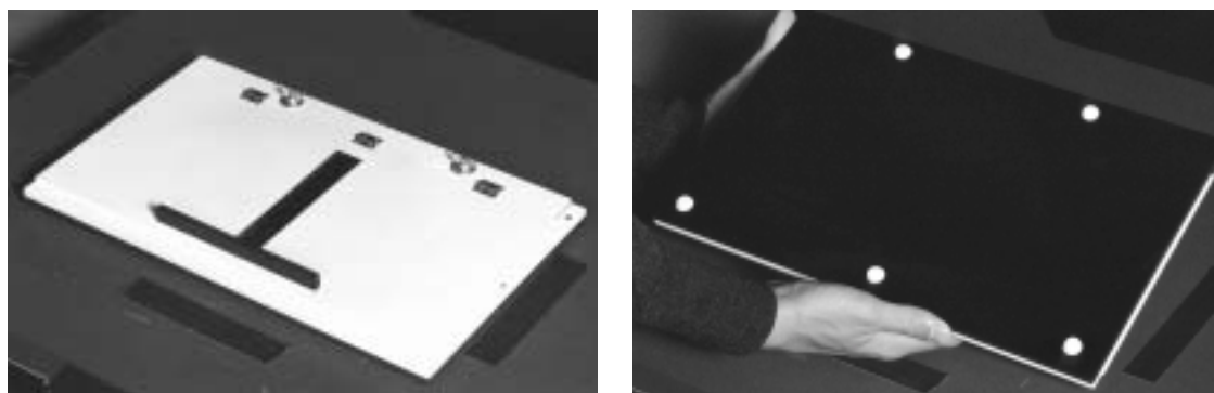
fig.6a-b The final test strip printer assembly. Five rubber feet ensure that it stays in place during operation and test exposures.
