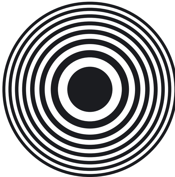
fig.19 Photon sieves (top) and diffraction zone plates (bottom) are worthwhile alternatives to plain pinholes, but they cannot be cut or drilled like a simple hole. The best way of making them is to take an enlarged, tone-reversed design and photograph it onto high-contrast B&W film thus reducing it to the desired size. The two designs shown here have a center pinhole diameter of 25 mm. Using the equations above, photograph these designs with a focal length (f) from a lens-to-design distance (u), or a film-to-design distance (a), in order to reduce the patterns by a known magnification (m), and create the required size on transparent film.
