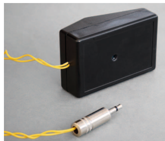
fig.2 The self-made shutter tester is connected to the microphone or line-in socket of a personal computer.
