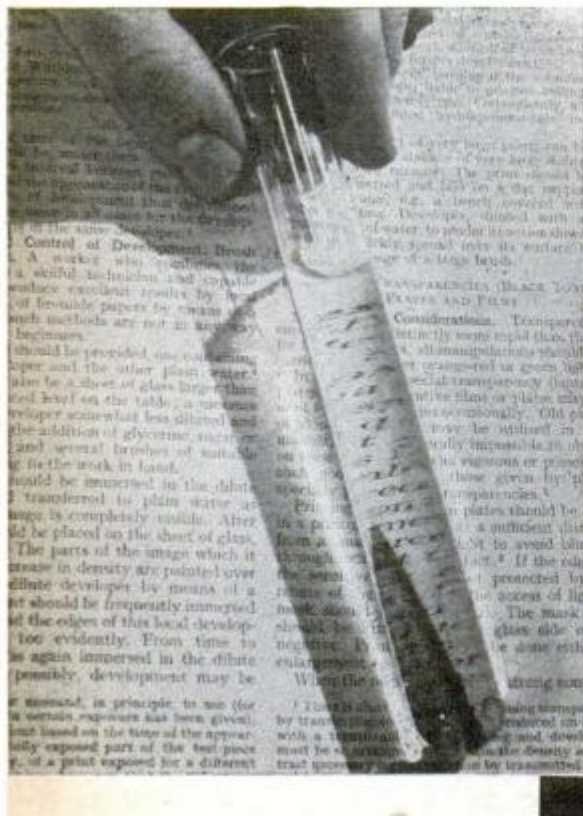
Fully developed black emulsion in the tube (left) becomes a clear solution when a reducer is added. That's how reducers act on overexposed negatives.
