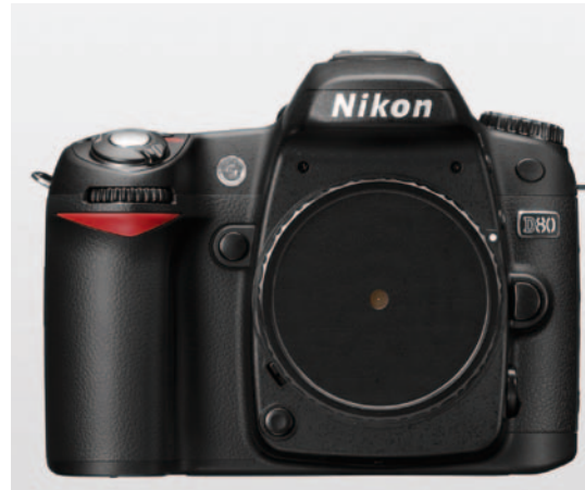
fig.8 Analog or digital SLRs are easily converted to sophisticated pinhole cameras by drilling a hole into a spare body cap and covering it with a pinhole plate.
