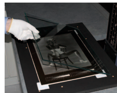
fig.6 In the darkroom, the digital negative is positioned, emulsion-side up, onto the paper and both are tightly held together by the weight of a thick sheet of glass. Subsequent exposure and paper processing are identical to analog contact printing.
