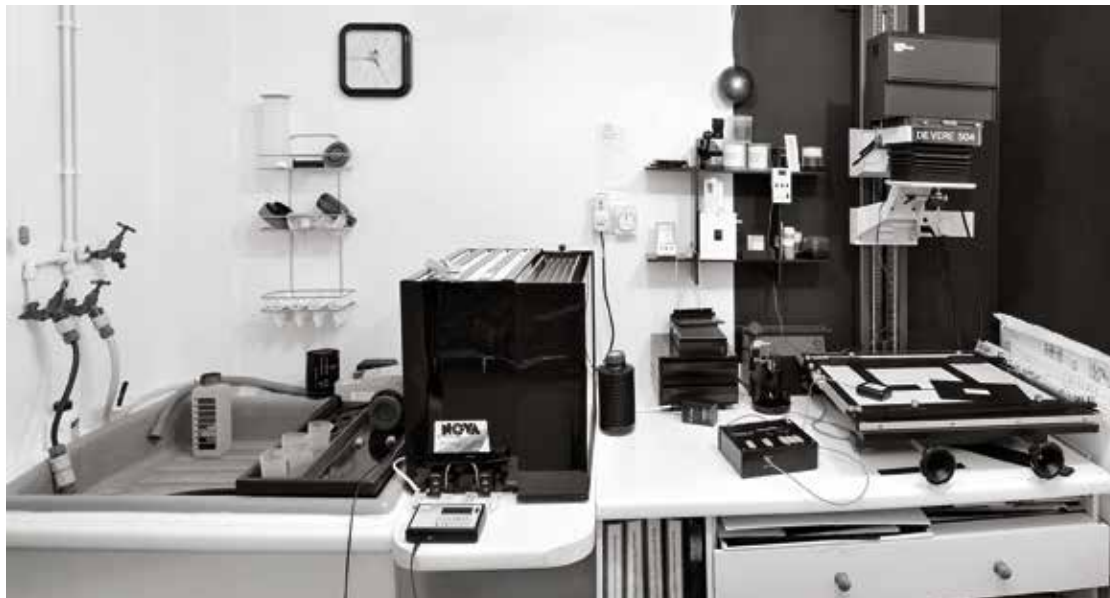
fig.10 (top) This medium-size darkroom in Ralph's basement offers a clear separation of wet and dry processes and ample space for tray processing. Multiple safelights are distributed throughout the room, and stray light from the enlarger is minimized by black curtains.
