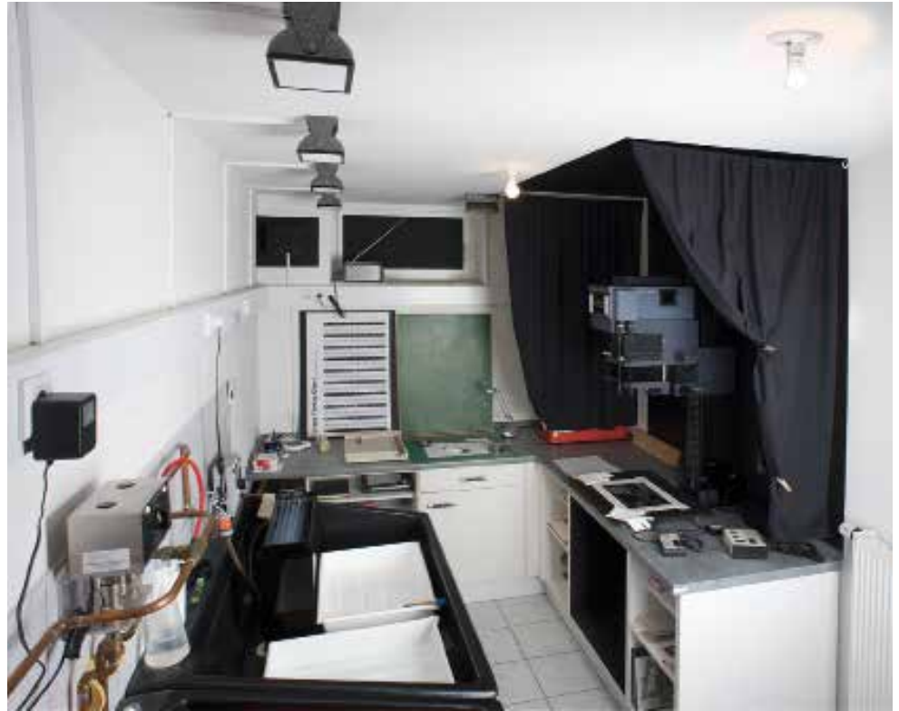
fig.10 (top) This medium-size darkroom in Ralph's basement offers a clear separation of wet and dry processes and ample space for tray processing. Multiple safelights are distributed throughout the room, and stray light from the enlarger is minimized by black curtains.
