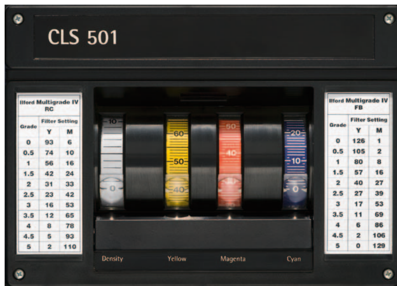
fig.2 A color enlarger with dichroic filters is a very useful piece of equipment for monochrome printing. The yellow and magenta filters can be used to fine-tune the paper contrast in VC papers, and even minute but precise contrast changes are simple by altering the two filter settings. A custom calibration allows precise paper grade settings in accordance with ISO standards.
