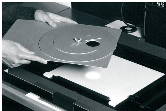
fig.4 The circular card in the center has several hole patterns to adjust the light path to specific applications. This light path can be further modified with the top card, by partially covering the chosen hole pattern. This way, many customized shapes are possible.
