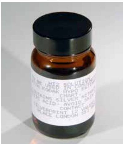
fig.11 Residual thiosulfate, left by the washing process, can be detected with Kodak's light sensitive silver nitrate solution HT2.
