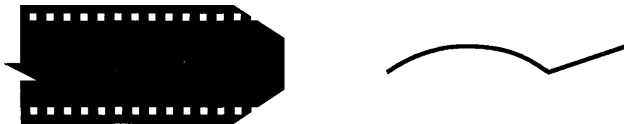
Figure 2 Left, cut off the corners of the leader to make it easier to thread the film through the camera module Right, make a reverse bend at the end of the leader to make it easier to feed the film into the take-up magazine
