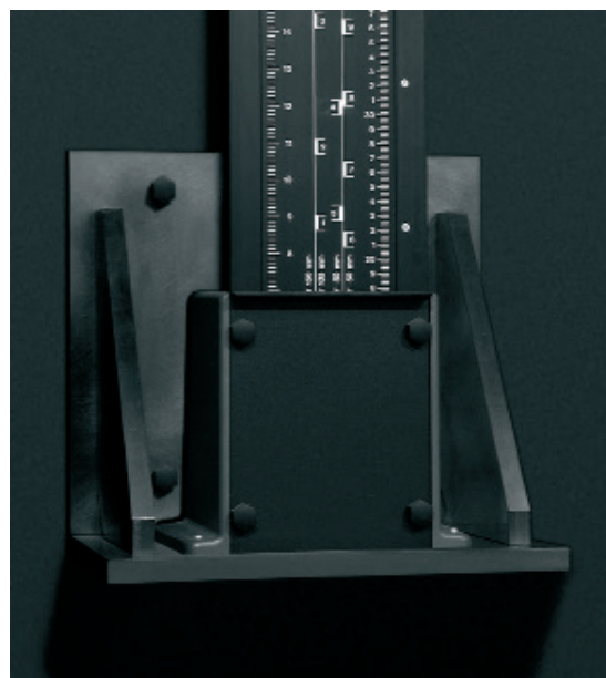
fig.1 (right) This professional Durst L1200 enlarger is wall-mounted through an aluminum bracket, which supports the enlarger's weight and isolates the column from vibration.
