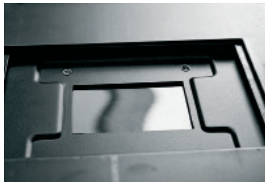
fig.3 This close-up of a glassless 35mm negative carrier clearly indicates an uneven film surface, seen in the reflection of a nearby window frame.
