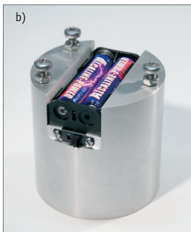
fig.5c The finished laser alignment tool is leveled on the baseboard and placed directly under the enlarger. The laser is then made to reflect off the negative carrier and the lens plane. The location of the reflected laser beam is a measure of misalignment.
